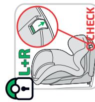
On the release buttons green safety indicators will be visible. Please check with the help of the safety indicators on BOTH SIDES, if the seat is properly connected with the two Isofix anchors (IA) of the car. The red markings must not be visible anymore.
