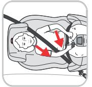
Now run the lap belt (**W**) with the lock tongue (**V**) over the armrests of the child car seat towards the three-point belt buckle and secure the lock tongue (**V**) from the three-point belt of the vehicle into the three-point belt buckle with an audible << click >>.
