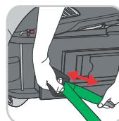
Press the release buttons. With an audible >> click << the ISO FIX Anchoring is unlocked. Now you can remove the child car seat.
